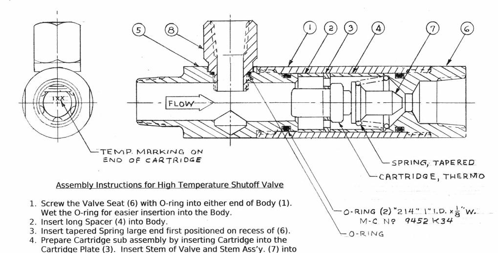
5. Verify that the Spring is properly in place, then carefully slide the Valve/Cartridge sub assembly into the Body (1) followed by the short Spacer (2).
